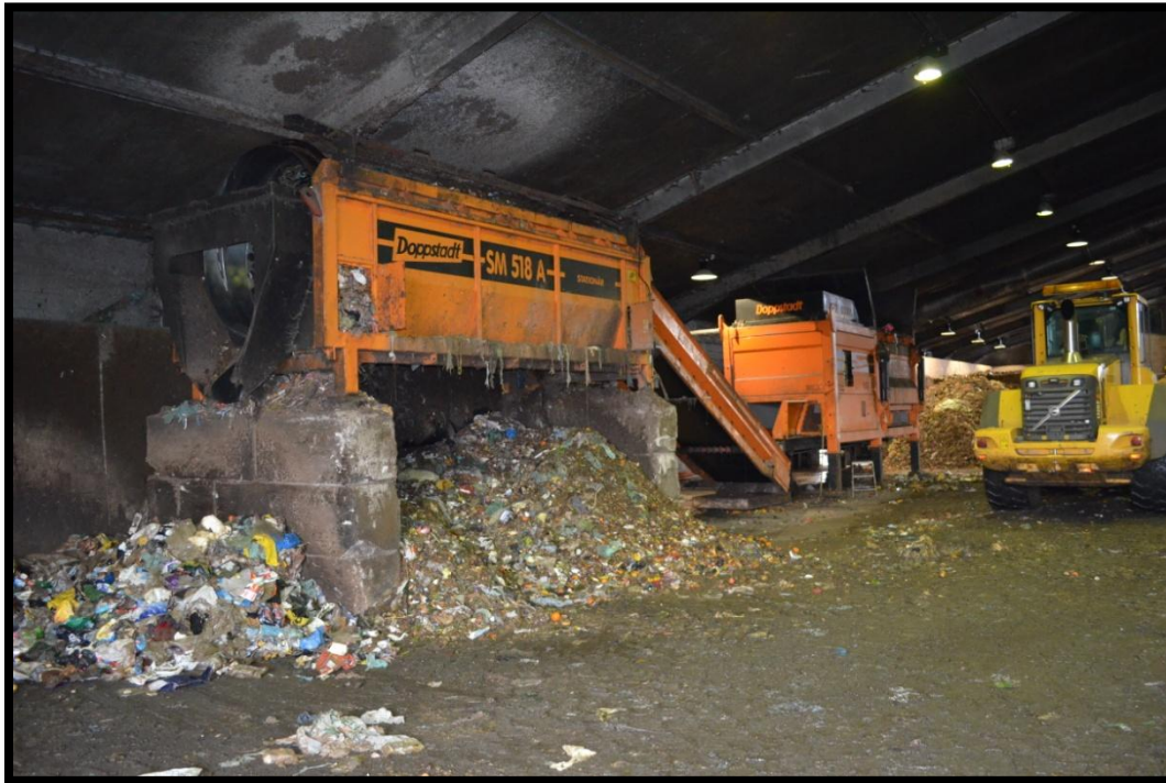
Figure 17: BioVækst's system for filtering plastic impurities
